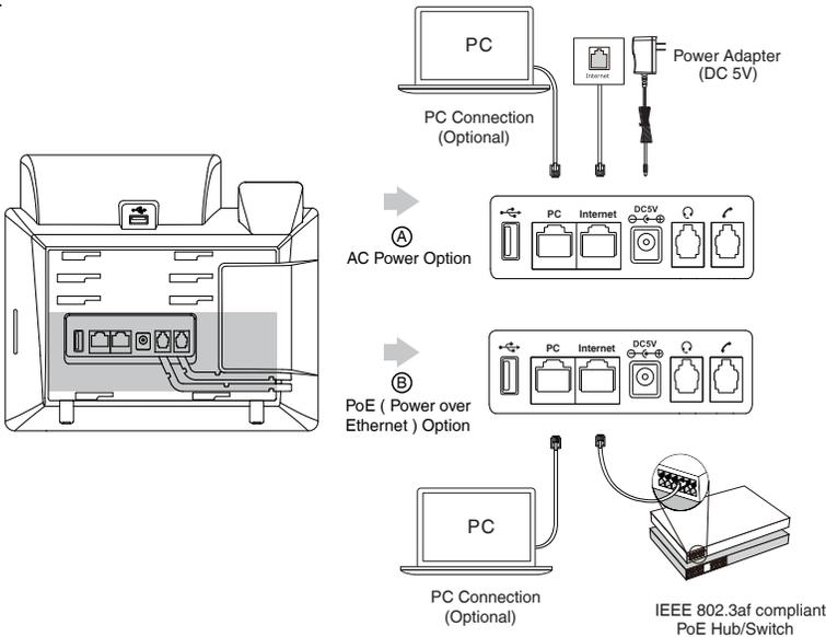
**Note:** The IP phone should be used with Yealink original power adapter (5V/2A) only. The use of the third-party power adapter may cause the damage to the phone. If you are connecting a PC to your phone, we recommend that you use the Ethernet cable provided by Yealink.
