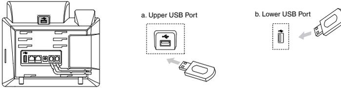
**Note:** The USB ports can also be used to connect other USB devices, such as EXP43, USB headset and so on. Yealink recommends that you connect Bluetooth USB dongle or Wi-Fi USB dongle to the upper USB port, and connect EXP43 to the lower USB port.
